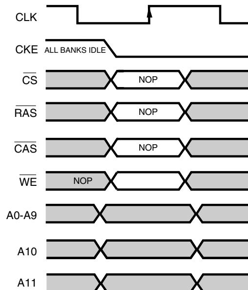
**Clock Suspend Command**
