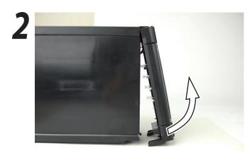
Lift up the front panel to remove it from the chassis.
