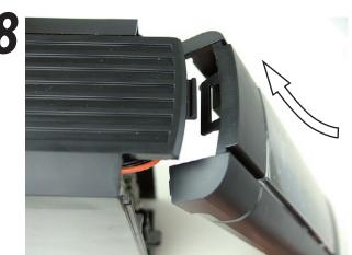
Insert the front panel, then secure it with the screw removed in step 1.
