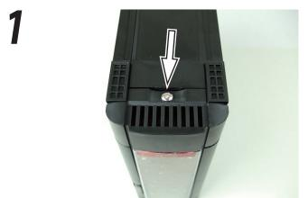
Remove a screw from the bottom of the KURO-BOX/PRO.
