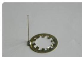
**Solder metal lead and bend to shape**
