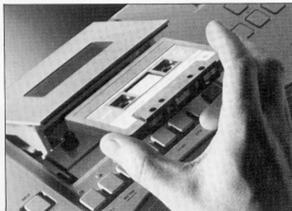
FIGURE 7. When inserting a cassette tape, make sure the open side of the cassette faces the front of your system.
