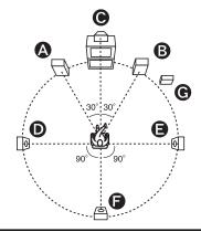
The front, center, and surround speakers should be placed at approximately the same distance from the seating area. The angles in the diagram are approximate.
