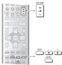
C (center), RS (right surround), SB (surround back) and LS (left surround) can be adjusted between -10 dB and +10 dB, with 0 being the level of the front speakers.
